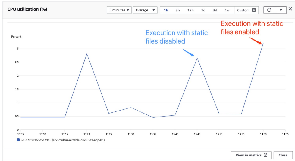
Figure 16: CPU utilization on EC2: 3 executions: the first and second has the setting '-blink-settings=imagesEnabled=false' and the third execution enables static files in the browser.
